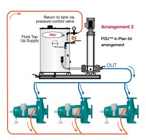
The diagram to the left illustrates how the FDU™ can supply multiple seal support systems. The diagram above illustrates how the FDU™ can supply multiple seals in a closed loop operation.
