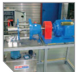
EDI Test rig for Pump packing
